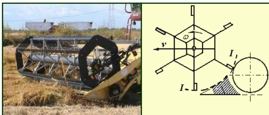
Graph 3: Computer model of harvester reel movement
