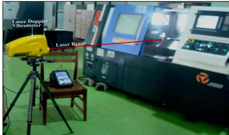
Figure 6 :Measurement of rotating work piece vibration using LDV
