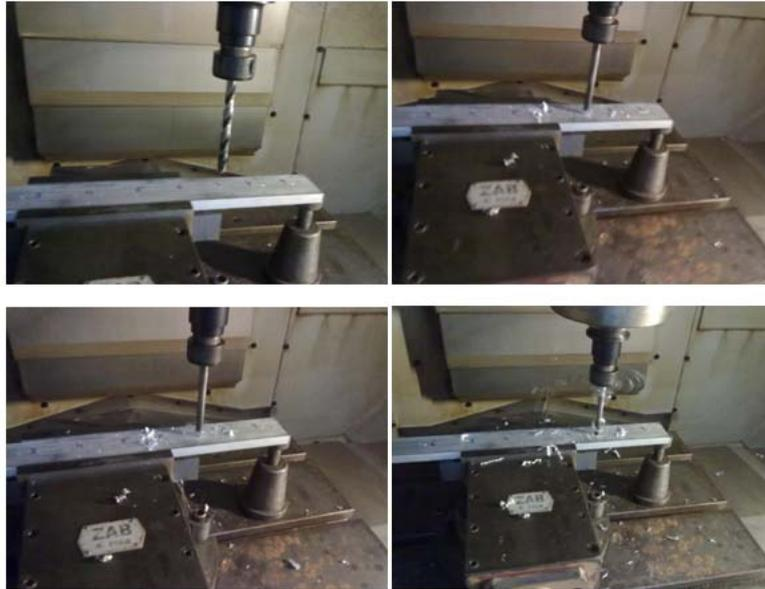
Figure 1: Drilling of Aluminum alloys
