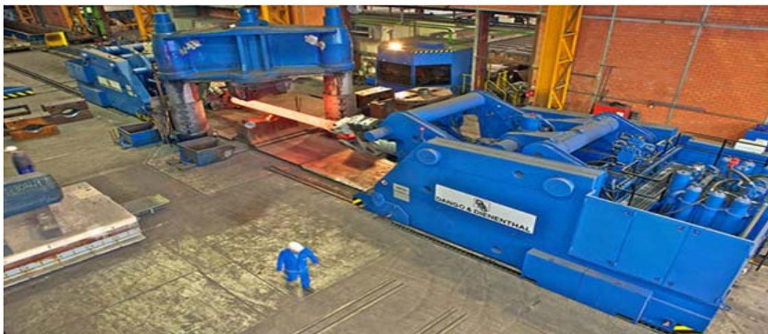
Figure 3: Forging Manipulator (Rail Mobile)
