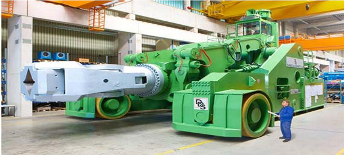
Figure 7: Forging Manipulator (Independent Mobile)
