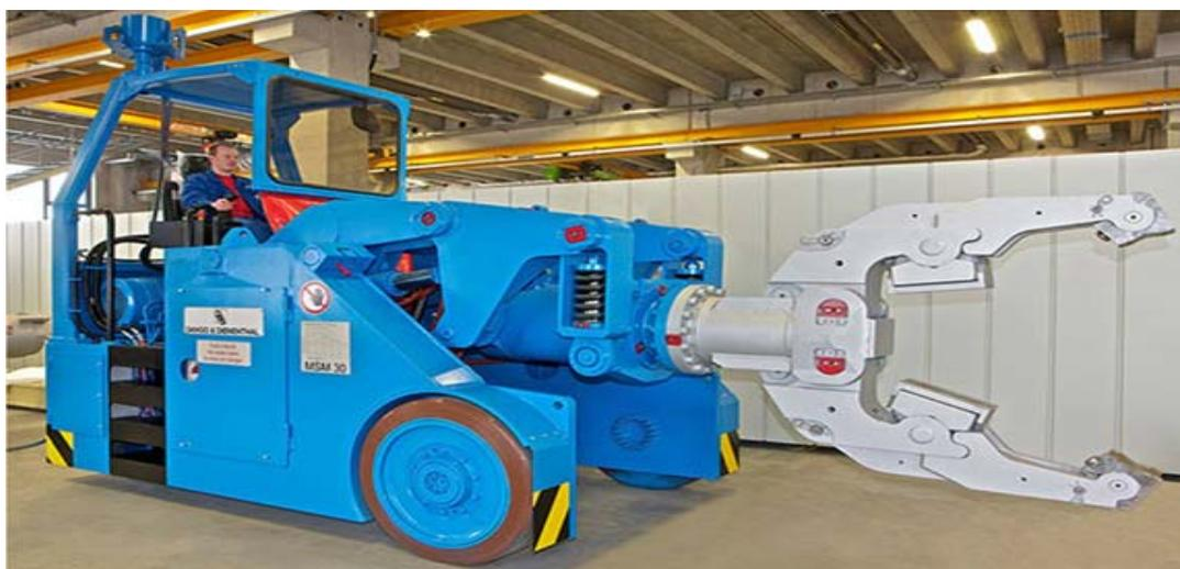
Figure 9: Forging Manipulator (Independent Mobile)
