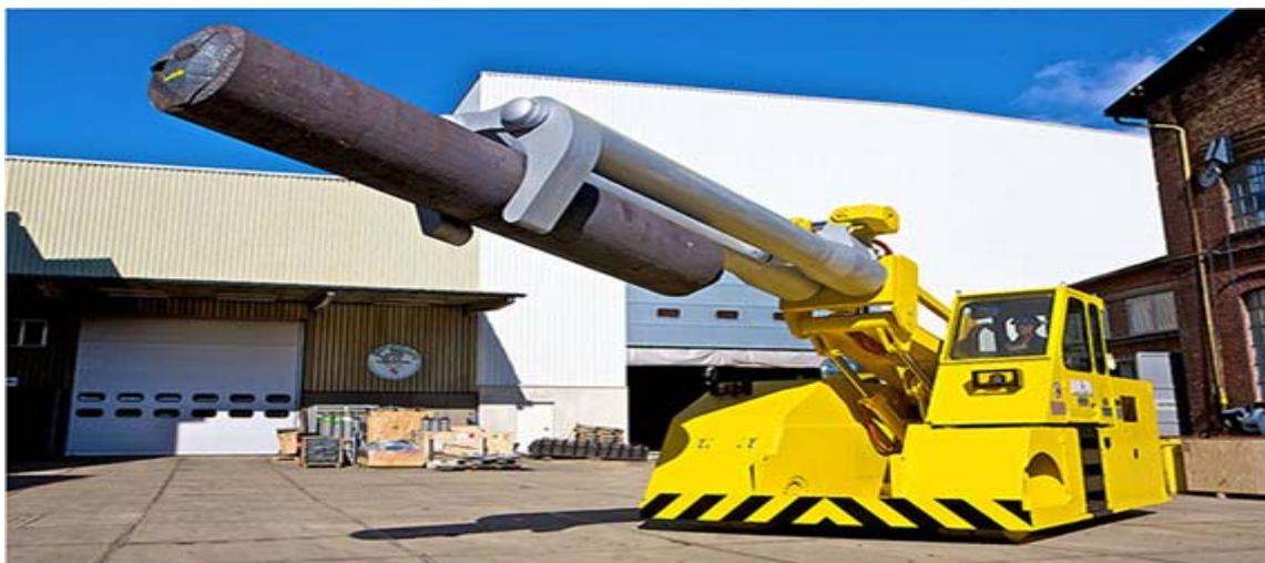
Figure 11: Forging Manipulator (Independent Mobile)
