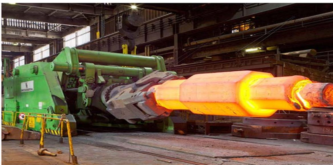
Figure 6: Forging Manipulator (Rail Mobile)
