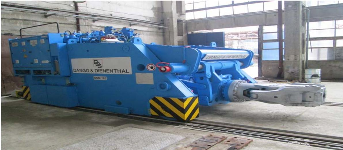
Figure 13: Forging Manipulator (Rail Mobile)
