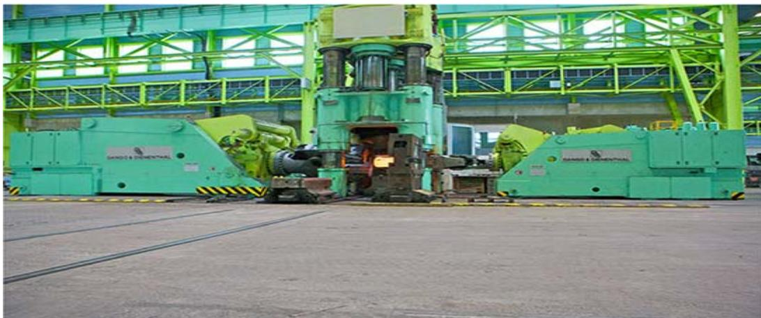
Figure 2: Forging Manipulator (Rail Mobile)
