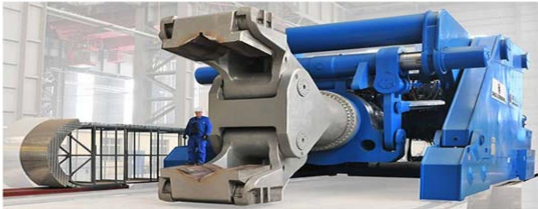
Figure 1: Forging Manipulator (Rail Mobile)
