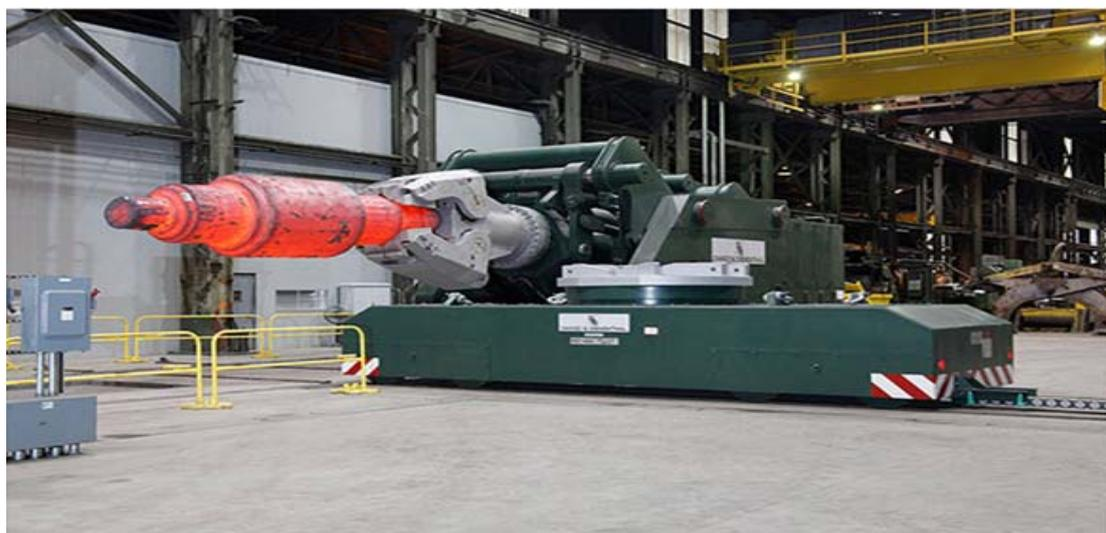
Figure 12: Forging Manipulator (Rail Mobile)
