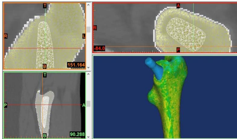
Figure 7: Assembly and material properties definition associated to the patient femur cortical and trabecular bone densities and to the Titanium prosthesis
