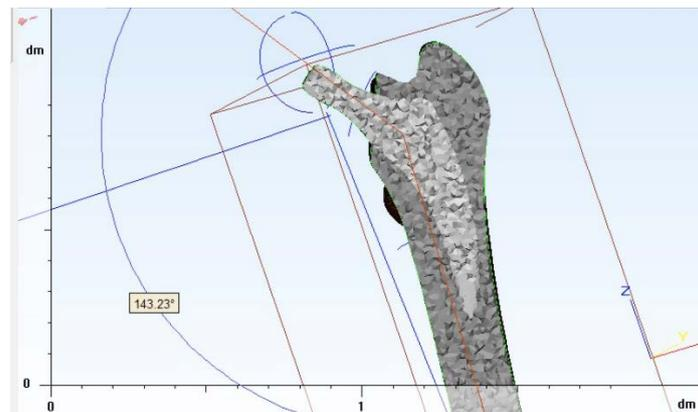
Figure 8: Assembly of the resected femur and Titanium rigid hip prosthesis and tetraedric mesh congruency verification
