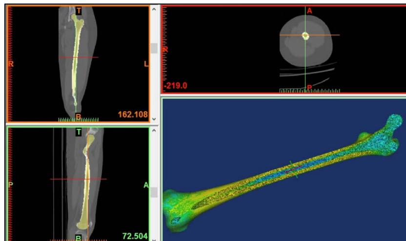
Figure 4: Mesh creation and optimization of the biofidel not resected femur model
