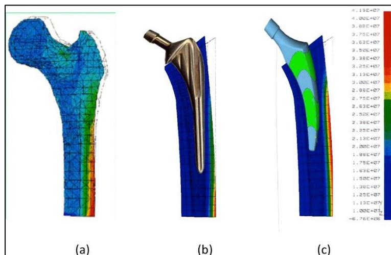
Figure 16: Equivalent Von Mises stresses distribution in the proximal femur epiphysis for (a) sound femur, (b) rigid Ti prosthesis and (c) flexible trabecular prosthesis
