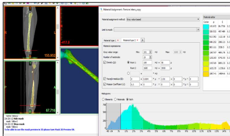
Figure 21: Material properties definition associated to the patient femur cortical and trabecular bone densities (left) and material properties assignment to HU bone densities (right)
