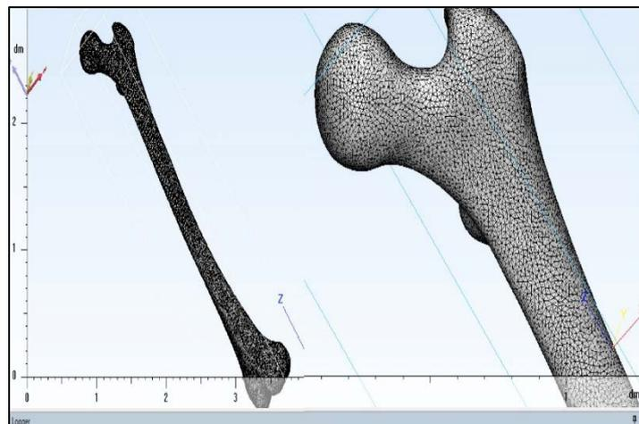
Figure 19: Preliminary triangle surface meshing optimization of the biofidel patient femur model
