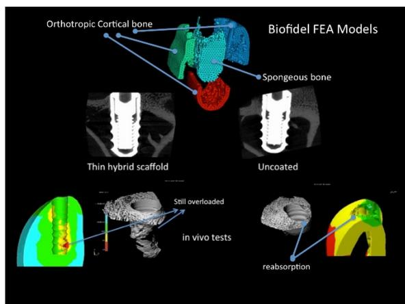
Figure 22: in silico and in vivo validation for Osteoconduction of Titanium implants coated with a nanostructured hybrid osteoactive (left side) and without (right).
