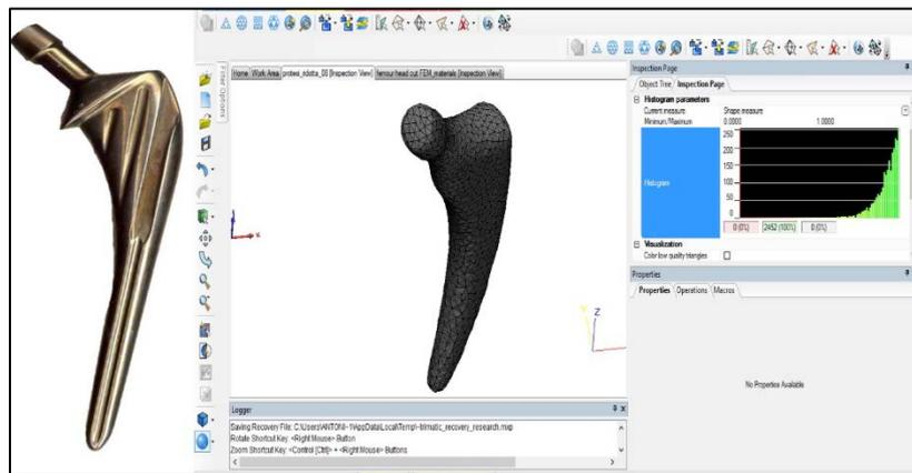
Figure 12: 3D meshing optimization of a Titanium traditional prosthesis
