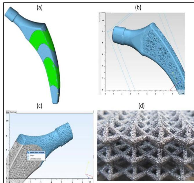
Figure 14: Flexible trabecular hip joint prosthesis with different stem and head rigidities and orientations. (a) Region of equivalent stiffness, (b) the overall flexible prosthesis, (c) internal trabecular structure, (d) Orthotropic trabecular structure obtained by additive sintering of Ti powders
