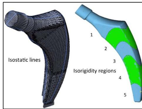
Figure 13: Left, Isostatic lines (Kummer, 1986) and right, Isorigidity regions chosen for the biomimetic prosthesis trabecular structure design
