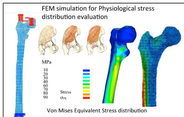
Figure 9: Physiological Equivalent Von Mises stresses in the femur from our biofidel Finite Element Model
