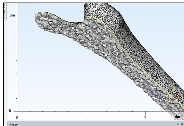
Figure 20: Tetrahedric 3D solid meshing optimization of the biofidel patient femur model (detail of the proximal end)
