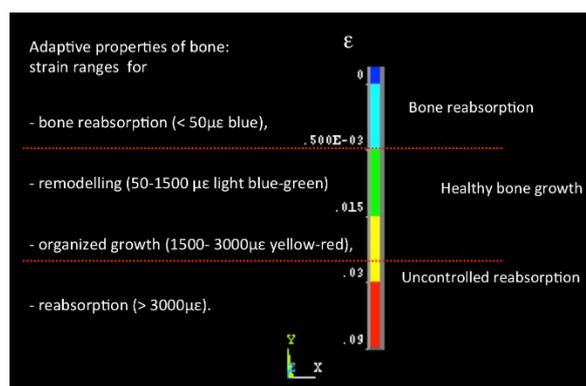
Figure 23: Frost (1990) adaptive window of bone physiology: Structural adaptations to mechanical usage
